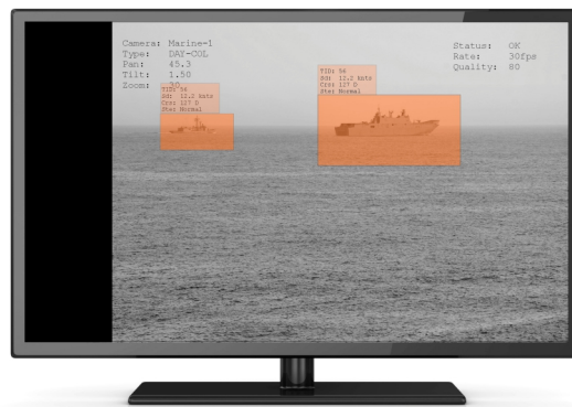
Figure 2: The video from the camera is overlaid with relevant target-specific data derived from the radar and other sensors.
